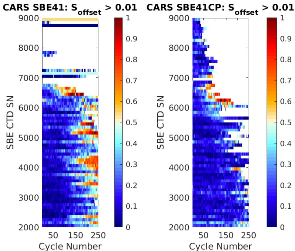
Figure 5 Fraction of assessed floats where the assessed salinity drift is greater than 0.01, as a function of cycle number. Bins for which there were less than 5 floats are omitted. The reference climatology is CARS. Left is for the SBE41 and right for SBE41CPs.
