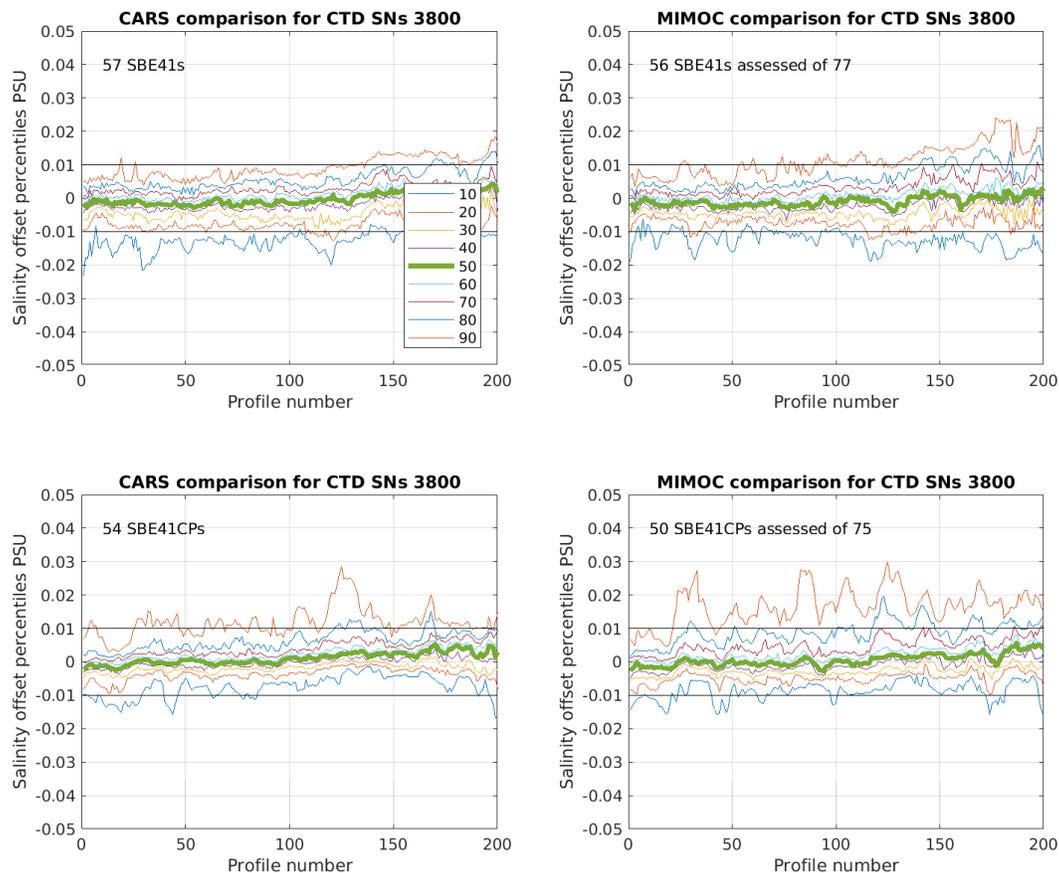
Figure 3 Percentiles of  $\Delta S$  as a function of cycle number for SNs between 3800-3899 for the two CTD types (top - SBE41s , bottom - SBE41CPs ) and for the two climatologies used to form the offsets (CARS left and MIMOC right). The total number of CTDs found is noted along with the number assessable.
